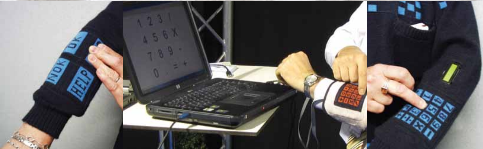
smart sweater with built-in battery recharge & textile keyboard connected to PC for read-out
