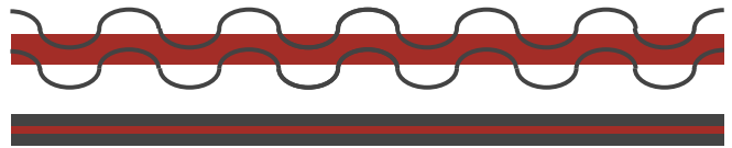
laminated textile or plastic layers (red = adhesive layer between two layers)
