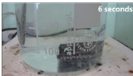
Carpet consisting of pile material and a bitumen backing. The design of the product is such that both parts of the carpet are separated within less than a minute when put into in boiling water.
