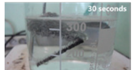
Carpet consisting of pile material and a bitumen backing. The design of the product is such that both parts of the carpet are separated within less than a minute when put into in boiling water.
