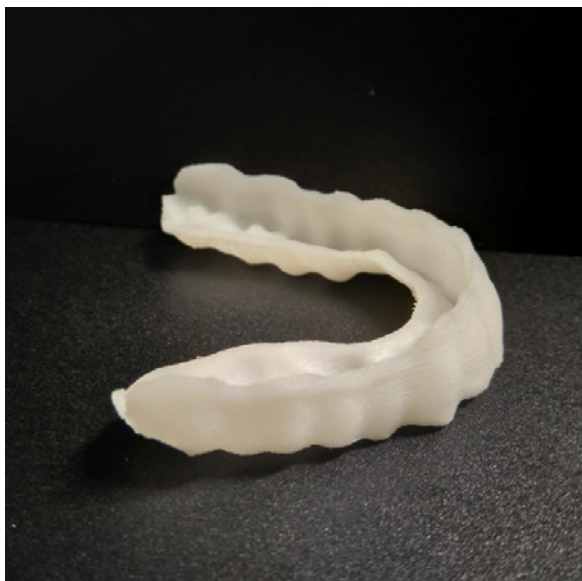
3D-print from a dental scan, printed with TPE, more specific TPS (Styrenic Block Copolymers), with a hardness of 90 Shore A.
