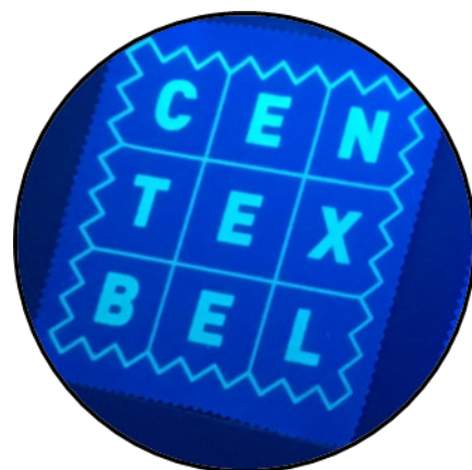
Screen printed textile with marker. Excitation with UV light
