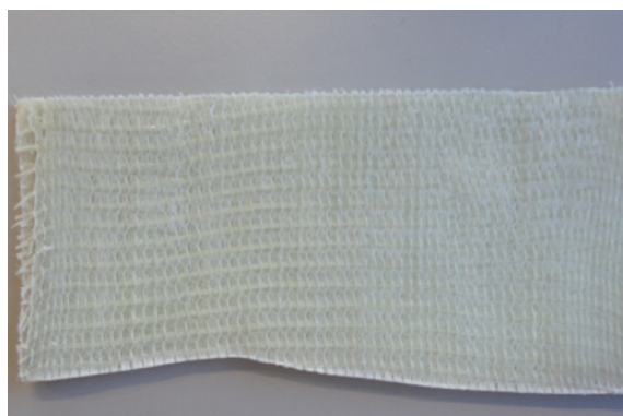
UV-LED cured composite (3mm thick)
