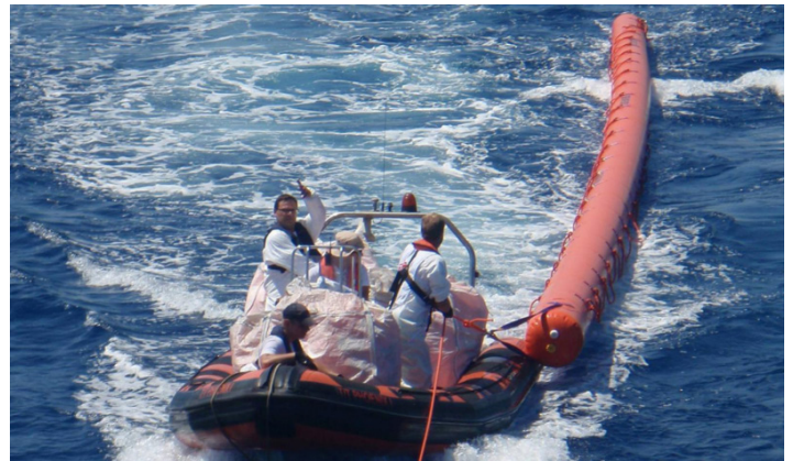
The Centifloat is a 16-metre, tube-shaped float, with more than 60 grab handles that can be inflated in three minutes and thrown over the side of high-sided container ships and ferries (Gabriele Francois Casini/MSF)
