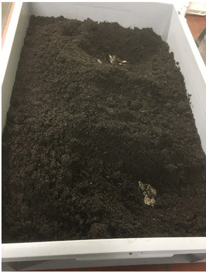
Soil burial test PLA coatings are buried to assess their degradability
