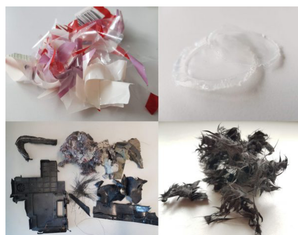
From waste to new materials - treatment of end-of-life flexible films and automotive scrap yield high purity mono-polymers and recovered reinforcing fibres
