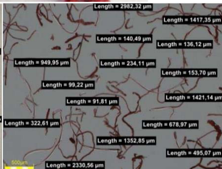
Images of the PES fibres granulated by Procotex including the determination of the granule size and fibre length.
