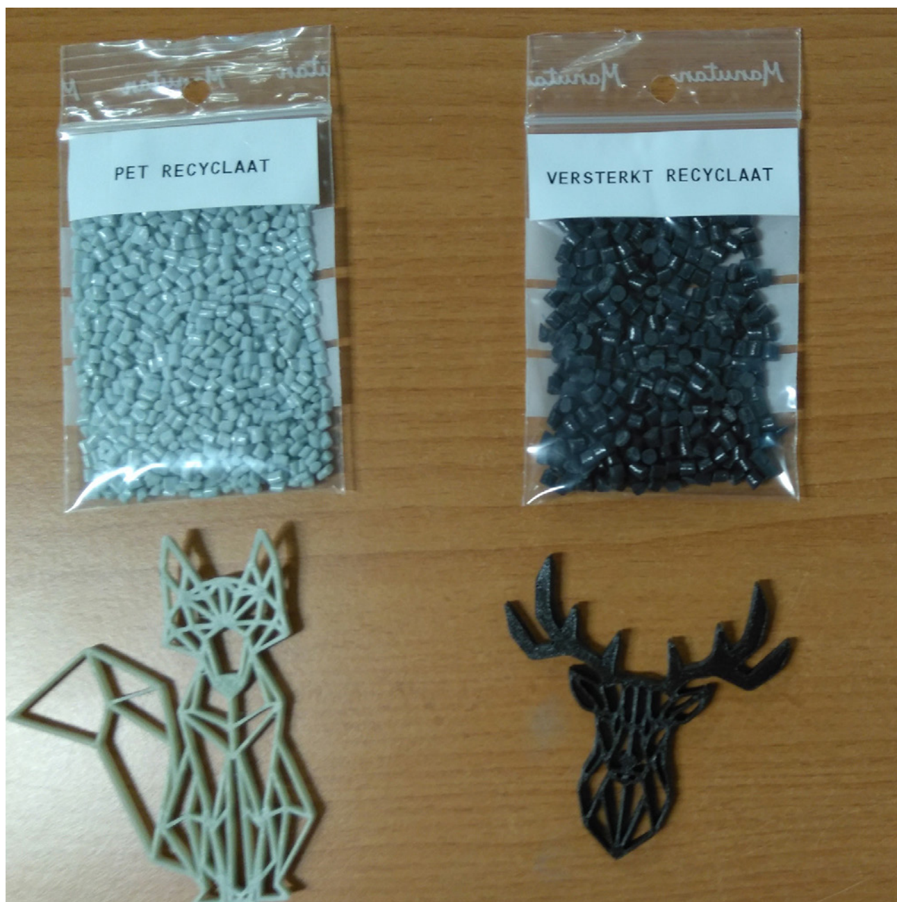
Figure 2: recycled materials after compounding/pelletization, and used in an additive manufacturing step
