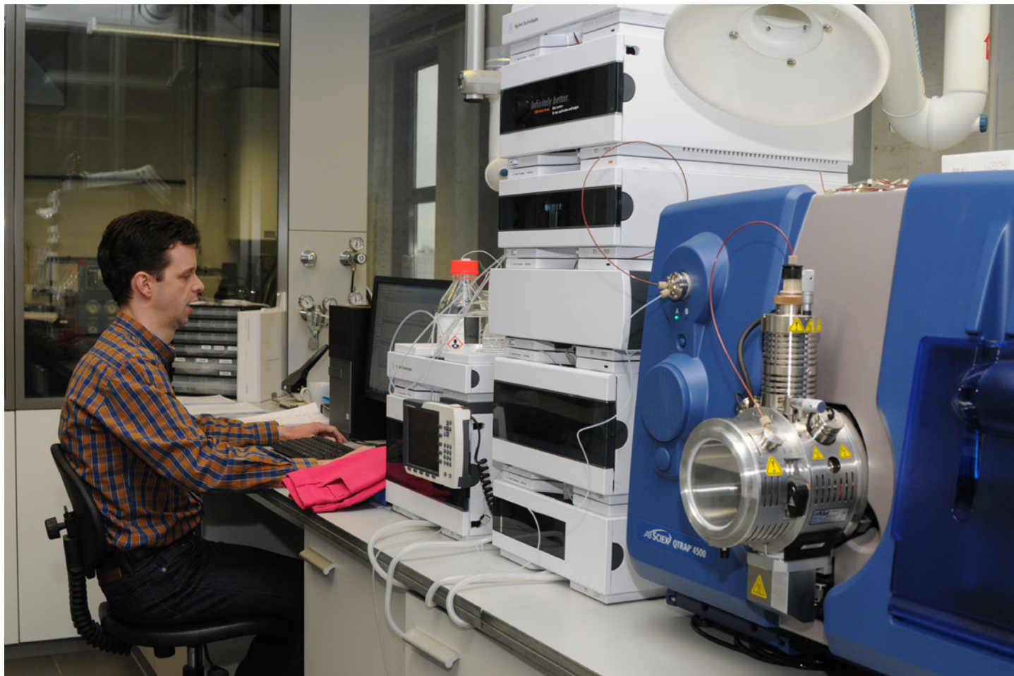
Centexbel is equipped to determine extremely low concentrations that amply meet the strictest legal requirements for the detection of chemical components in materials. Photo: HPLC/MS device operated by David Van de Vyver who developed the test method for OEKO-TEX®.
