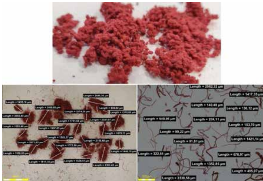
Images of the PES fibres granulated by Procotex including the determination of the granule size and fibre length.
