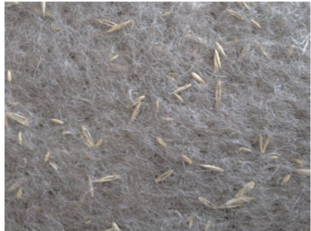
PLA non-woven felt with grass seed incorporated in 3D structure - demonstrator - DS Textiles
