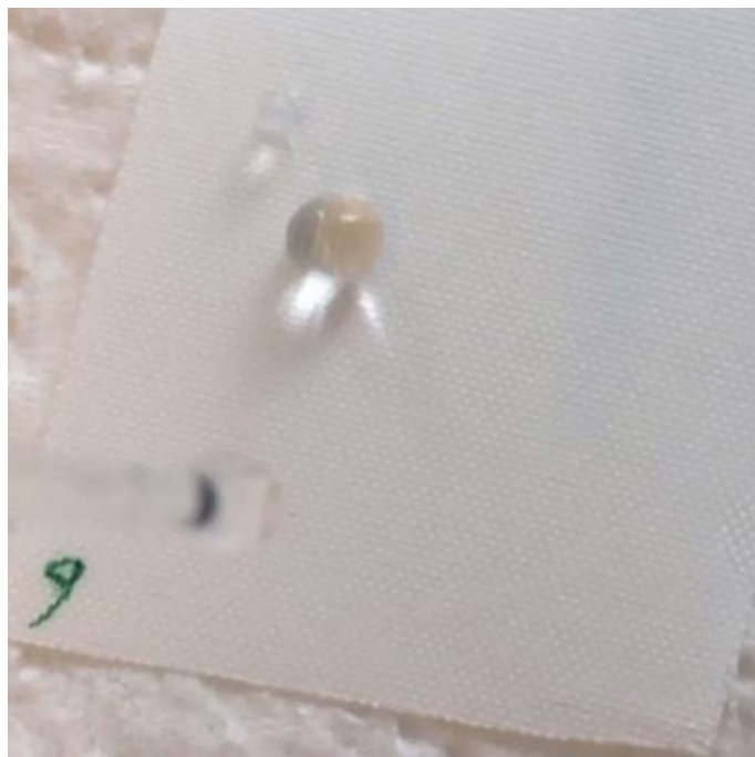
Water droplets rolling off a superhydrophobic polyester fabric
