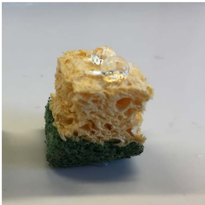
Water droplets on top of a cellulose sponge treated with a superhydrophobic fluor-free formulation
