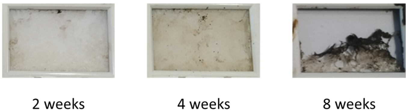
Figure 7. Disintegration of PU films made with 1% crosslinker, after 2, 4, and 8 weeks.
