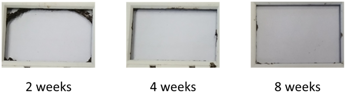
Figure 6. Disintegration of non-cross-linked PU film after 2, 4, and 8 weeks.
