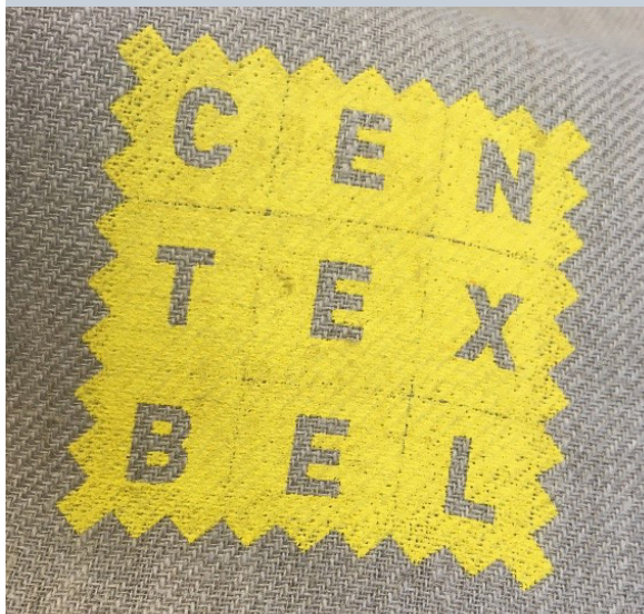
Picture 3: A screen-printing ink based on polylactic acid, they are mildly washable at 30°C and do not contribute the microplastics as it is mixed with highly biodegradable eco-friendly plasticisers.
