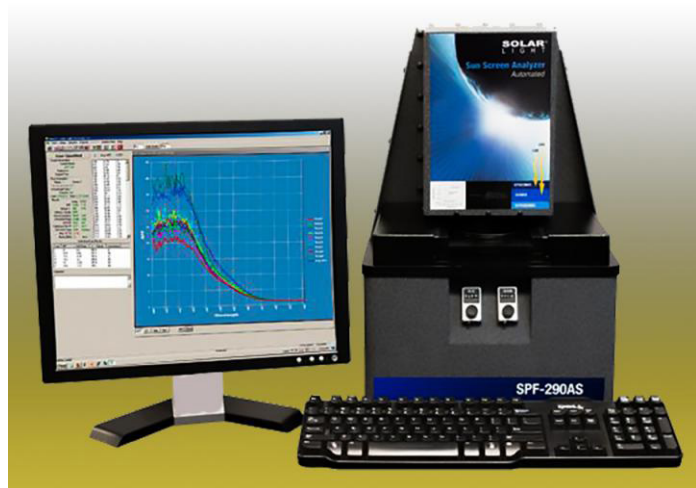
The tests were performed on the Solar Light's Ultraviolet Protection Factor (UPF) Analyzer, SPF-290AS
