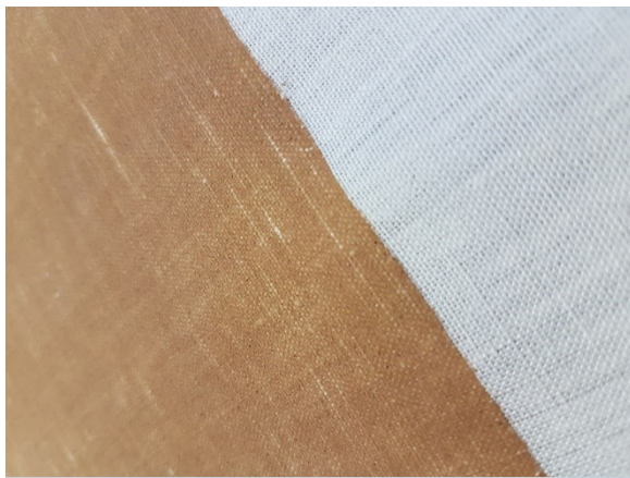
Picture 1: This 100% bio-based and fully biodegradable coating uses a polymer produced by bacteria as binder and has cork as a filler material, giving the coating a velvety touch.
