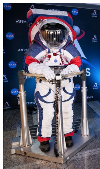
NASA's new EVA suit provides improved range of mobility. Source | NASA
