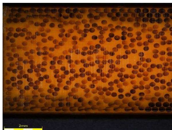
Figure 2: fibres and matrix of SR-PLA after compression moulding
