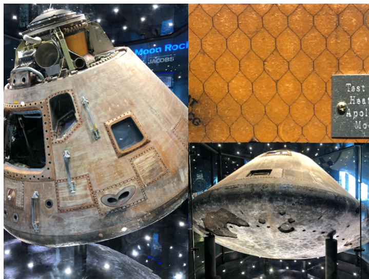
Apollo's heat shield was made of epoxy phenolic novolac resin in a fibreglass honeycomb. © CW photos | Scott Francis
