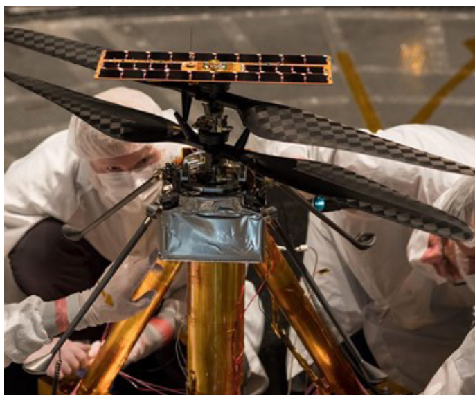
More than 1,500 individual pieces of carbon fibre were used in the construction of the Mars helicopter. Source | NASA
