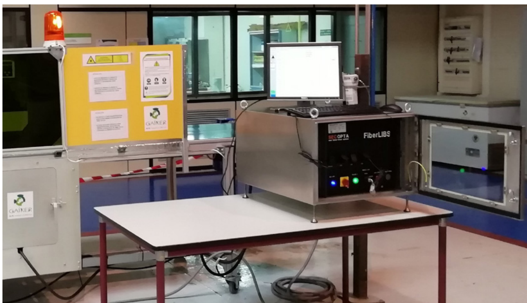
LIBS technology to sort bromine-contaminated plastics
