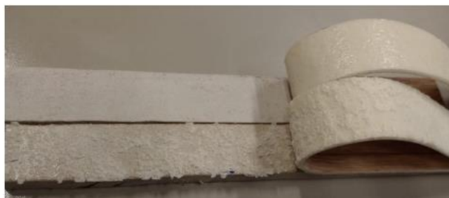
Figure 57: Results from the experiments – Top) PSA sample, Bottom) commercial tackifier sample
