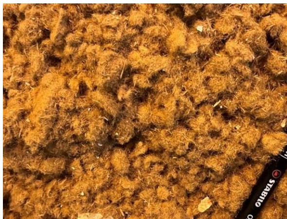
Figure 4: Recycled fibers from EoL laminate flooring containing coating flakes (white)
