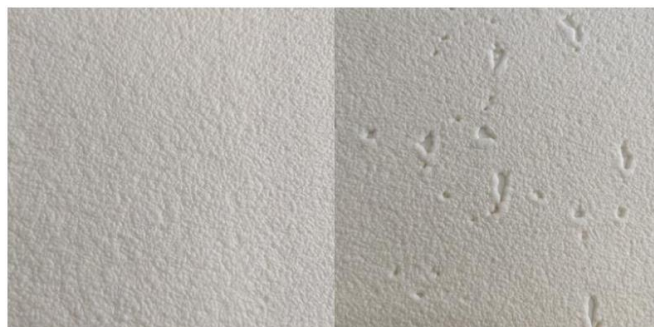
Figure 51: Reference vinyl product (left), holes appeared in the back foam with recycled content during the edge trial (right)
