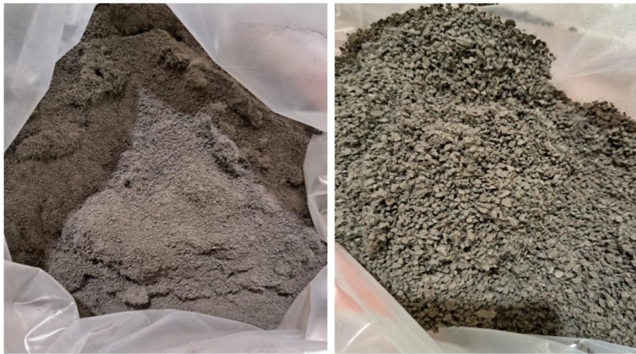
Figure 37: Two images of small samples of sieved backing stream. On the left, the fraction with lower particles size distribution, on the right the coarse fraction.
