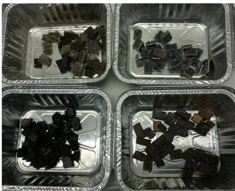
Figure 30: Outcome reactions on carpet tiles: Left top) bitumen backed in alcohol, Left bottom) bitumen backed in acidic conditions, Right top) polyolefin backed in alcohol, Right bottom) polyolefin backed in acidic conditions
