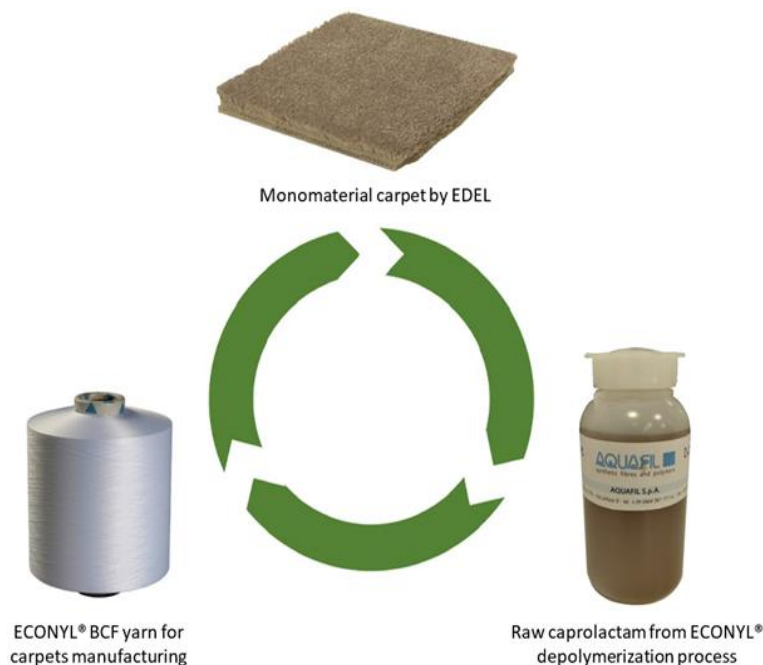
Figure 25: Schematic summarization of the circularity of monomaterial carpet
