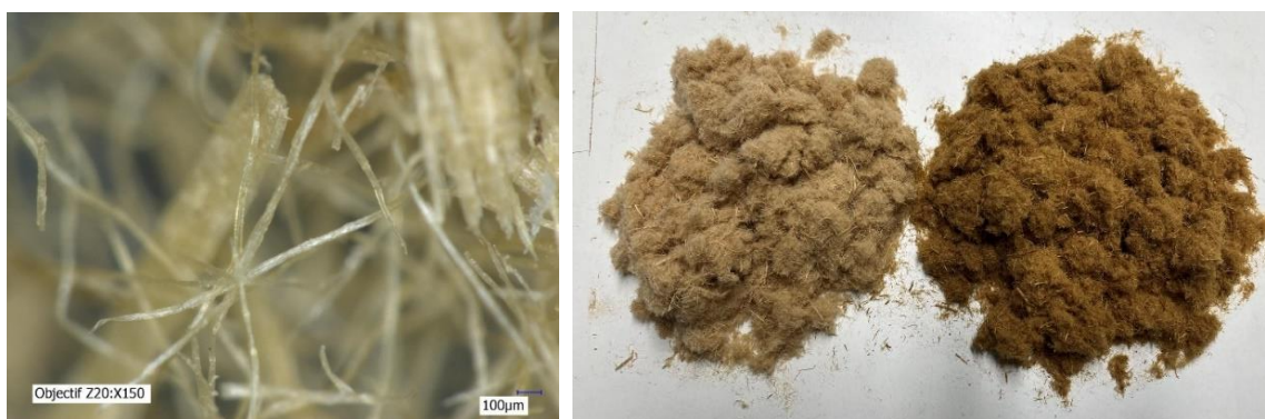
Figure 5: Left) Optical microscope of recycled fibers showing smooth and intact fibers surface, Right) Left: virgin fibers - Right: recycled fibers
