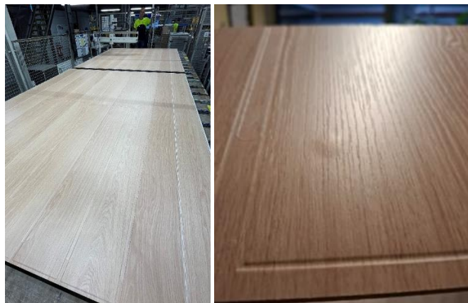
Figure 9: Circular laminate flooring production (left) and a small defect (bump) on a laminate flooring plank (right)
