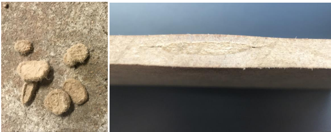
Figure 6: Fiber lumps (left) and effect of such a lump in a HDF board (X-section) (right)
