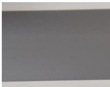
Figure 56: 100% recycled CV sheet obtained by the two-mill roll
