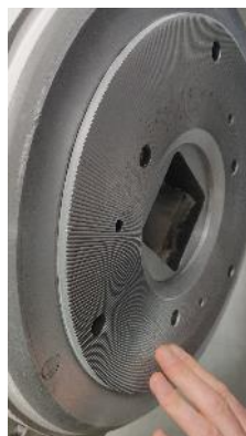
Figure 47: Pulverisation disk inside a microniser
