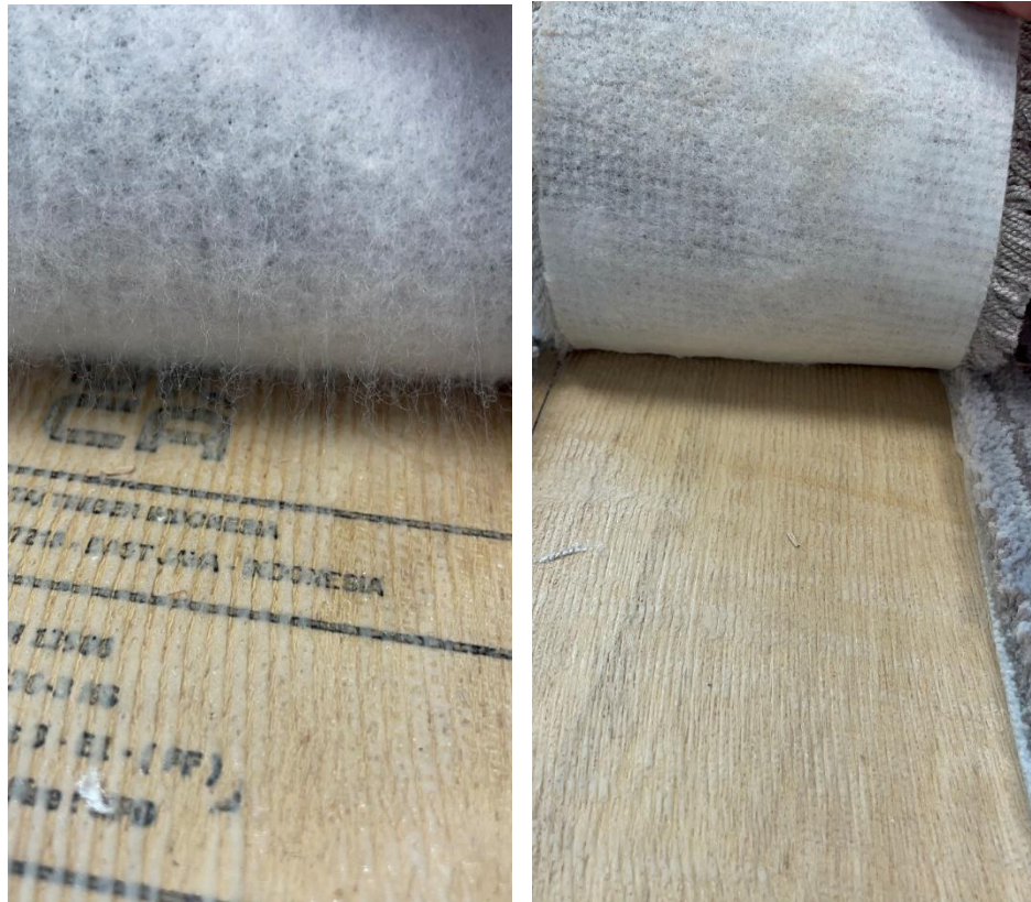
Figure 21: Original cTextile backing sample (left) and modified cTextile backing (right)
