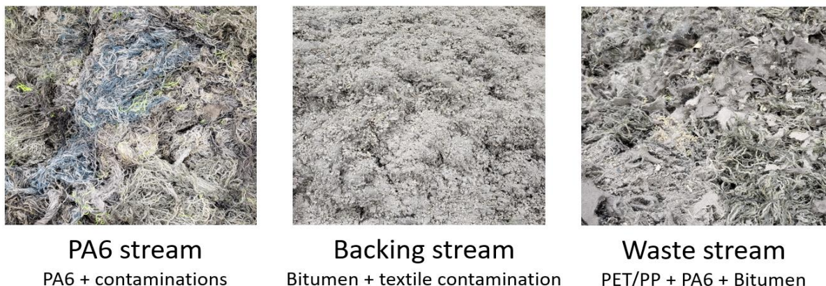
Figure 40: Like bitumen-backed carpet tiles, also PO-backed ones when processed divide into three streams.
