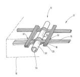
Because of the direct connection between the fastening element (12 to 15) and the reinforcement (17), the prefabricated concrete element can have an especially extensive and thin form and thus can be used as a façade panel.
