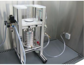
BFE test – developed by Centexbel
