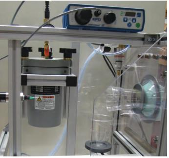
Splash resistance test - developed by Centexbel
