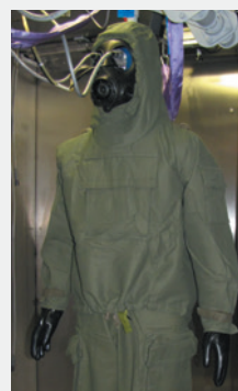
ASTM F2370 standard test method for measuring the evaporative resistance of clothing using a sweating manikin
