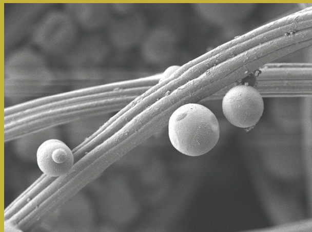
mattress ticking with incorporated PCM for thermoregulation
