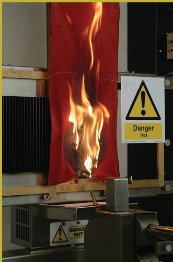
example of rapid vertical flamespread and hence poor burning behaviour
