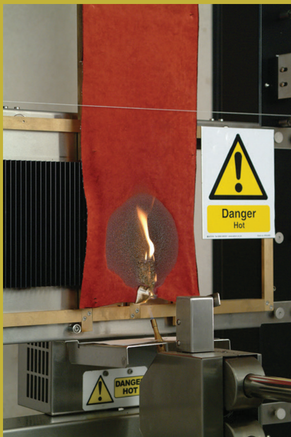
example of rapid vertical flamespread and hence poor burning behaviour
