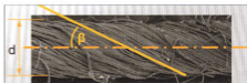
Fig. 5: flax yarn showing the mean angle of the fibres to the yarn axis \beta . This angle should be minimised in composite preforms 1 .
