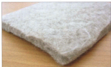
Fig. 4: flax/PLA air laid and needle punched nonwoven
