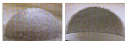
Fig. 7: formed and consolidated nonwoven. The figure on the right shows the importance of controlling the clamping force to achieve the desired thickness, with a thinner cross section in the centre of the dome.
